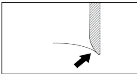
**Important:** the inner edge of the upper cut must be well rounded
