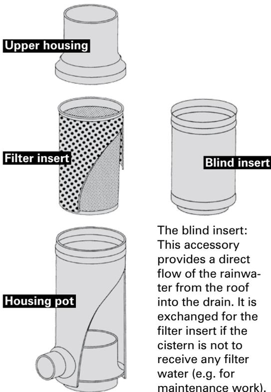
The blind insert: This accessory provides a direct flow of the rainwater from the roof into the drain. It is exchanged for the filter insert if the cistern is not to receive any filter water (e.g. for maintenance work).
