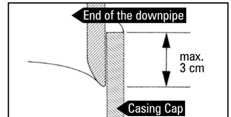
– It is important to match the filter size with the correct pipe diameter. The top cap of the filter is designed to be a dose fit on the pipe to ensure that water flow is directed over the surface of the filter element.
